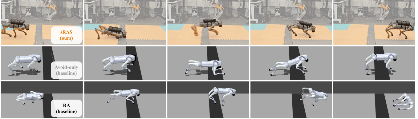
Fig. 1. A Unitree Go2 quadruped must jump across a 25 cm gap, land safely on the far side, and remain safe afterward. This is a strict reach–avoid–stay ( sRAS ) task, where a robot must safely reach a target and remain safely within it indefinitely after first target entry. All methods use the same task policy, which is a pure-pursuit policy that walks in the right direction. Sequences progress from left to right. Top (hardware) : With our sRAS Q -control barrier function (CBF) safety filter, the robot builds momentum, crouches for takeoff, jumps across the gap, lands safely, and remains safe. The same successful behavior is observed in simulation. Middle (simulation) : The Avoid-only safety filter does not encode reaching the far side; the robot fails to complete the jump, leaving its hind legs on the starting side. Bottom (simulation) : The reach–avoid ( RA ) safety filter encodes reaching the target safely but not remaining safe afterward; the robot jumps across the gap but fails to land safely. The successful hardware execution illustrates the intended behavior of our sRAS Q -CBF filter: modifying task actions to keep the robot in sRAS winnable states and maintain safety within the target after first target entry.
